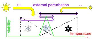
Figure 2: Black, white, grey daisies have same (green) viability dependence on local temp. External forcing from Sun varies. Black increases, white decreases local temp. Feasibility ranges (\iff ) of both B&W are extended to lower/higher perturbations.
